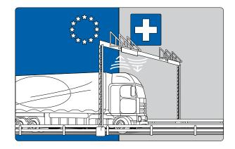
When entering or leaving Switzerland at the border, the OBU automatically establishes contact with radio beacons and calculates the chargeable tonne-kilometres.
