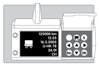
Foreign vehicle owners can voluntarily equip their vehicles with a Swiss HVF on-board unit (OBU). The OBU is installed in the towing vehicle and automatically records the distance covered.
